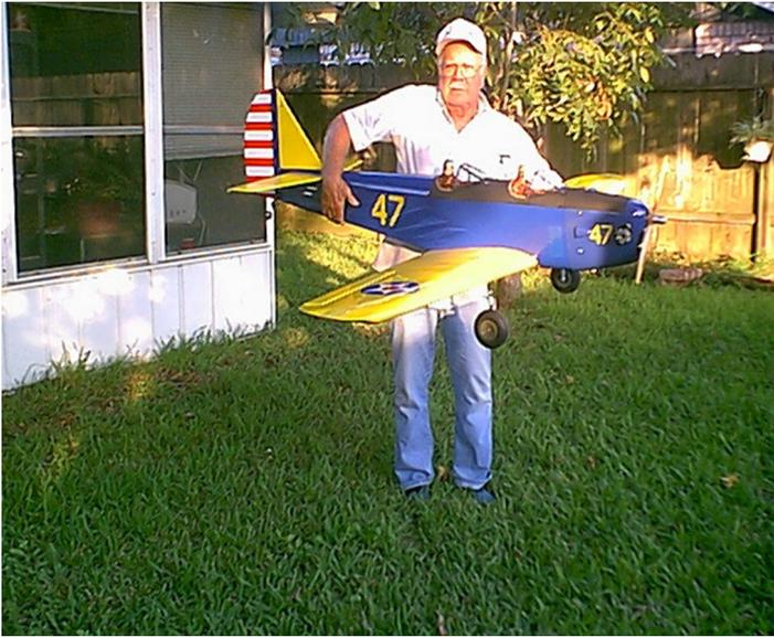
Don Fisher's PT 19 by Hanger Nine. It has one flight on it so far and flies well. It weighs 14 1/2 pounds and has an 81-7/8" wing span and has a Zenoah G38.
