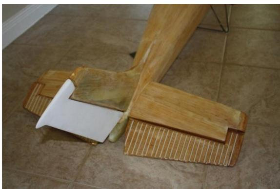
I used my heat gun to help remove the MonoKote leaving a lovely layer of white goo to remove before I could prep the surface to be glassed. In the process I also found out that the original builder had the same idea of fiber glassing but must have given up when the epoxy did not completely cure. After all these years the epoxy was still a little gooey/tacky. Add the leftover goo from the MonoKote and ailerons could second as quality fly-paper.
