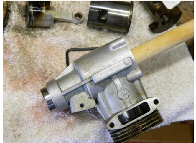
The front bearing can be tapped out with a dowel rod. Now it's time to heat up the crankcase and drop out the rear bearing.
