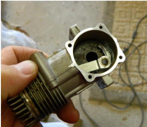
New bearings installed now just re assemble the engine. BTW the old bearings had a lot of play in them.
