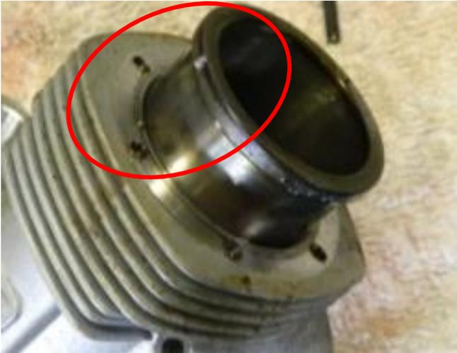
Once the cylinder sleeve is removed the piston rod may take a little coaxing to get off the crankcase. But once it is off the piston comes right out. If it is a ringed engine you must make sure the ring is in the correct position when putting it all together.
