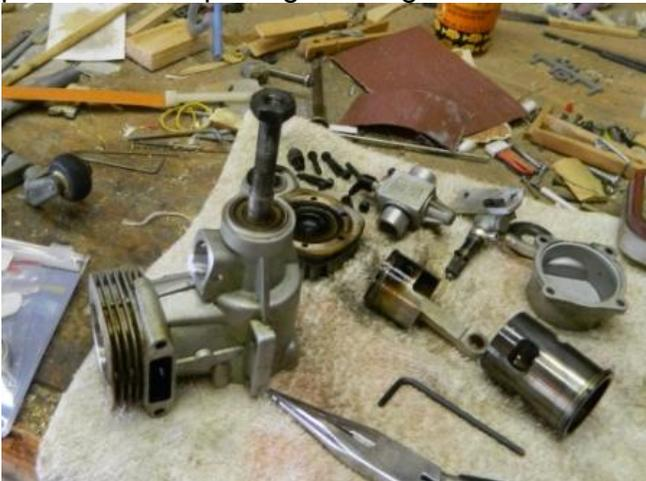
Once that is complete you need to tap out the crank from the old bearings. This can be done by tapping the nut on the shaft. No problem.
