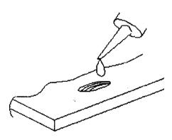
When you drill and tap holes for wing bolts and hold downs, adding some CA is a good way to add strength to the threads. After it sets up, tap again. If the
