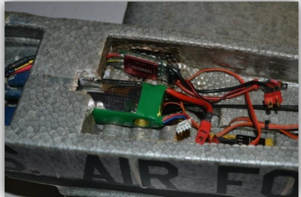
This is the stock battery mount for a Parkzone T-28. Mine eventually became loose enough to allow the battery to fall free in flight.
