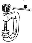
Removing the T-bar (arrowed) from your small C-clamps and force fitting a small piece of windshield washer hose to the threaded part allows the clamps to be used in confined spaces. Adequate clamping force can still be applied for hobby purposes. Ray Stark, Rancho Cordova, California
