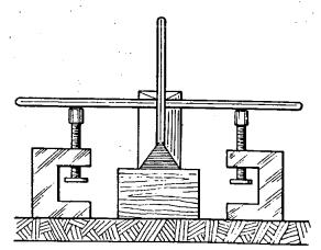
Your X-Acto clamps can also do double duty as levelling jacks when "squaring up" that new model. Use adhesive tape to hold them firmly to the bench and use them in conjunction with a bubble level.
