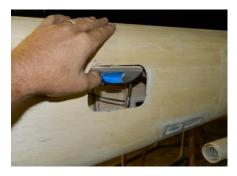
The next picture shows the fiberglass lay ups I made for life boat hatches. These hatches will cover the on-board glow drivers.
