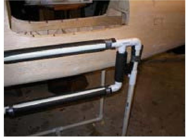
One last pic is of the cradle I designed. The arms shown in the pic rotate up and have a threaded bolt for stability. The wing can then be rested above the fuse, all connections made and then the arms can be rotated down and wing attached. As I always say, in theory it should work.
