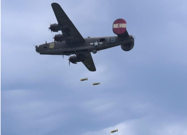
Bombs away. These are knew bombs. 3D printed by Fitz Walker and perfectly weighted by me. I used a ½ oz lead in the nose, filled with that expandable filler, and plati-dip the nose. They look great in the air.
