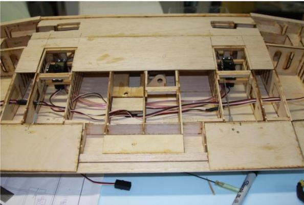
The fuselage comes with extensive cockpit details some of which are installed and painted early in the build. I can see that it had to be this way but I kept breaking some of the thin balsa parts every time I flipped the fuselage over.
