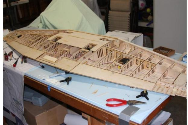
The wing has since been sheeted and is ready for final sanding. The modifications I made added some weight in exchange for some ease of maintenance and accessibility.
