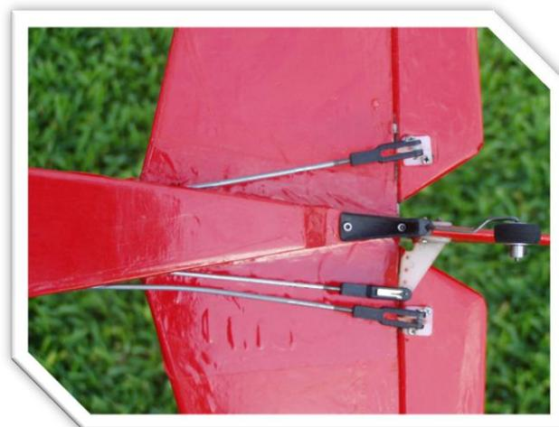
Upgraded tail controls. Heavy duty horns on elevator, heavy duty pushrods and 2 pushrods on elevator to eliminate twist in wire joiner.
