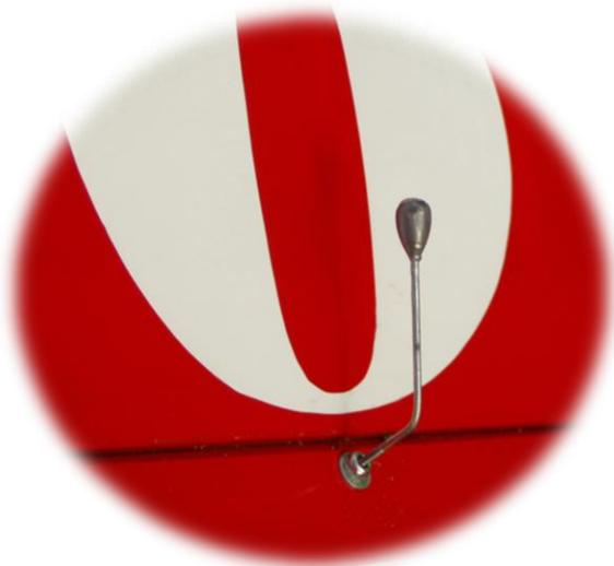
Aileron counterweights completed the equation.
