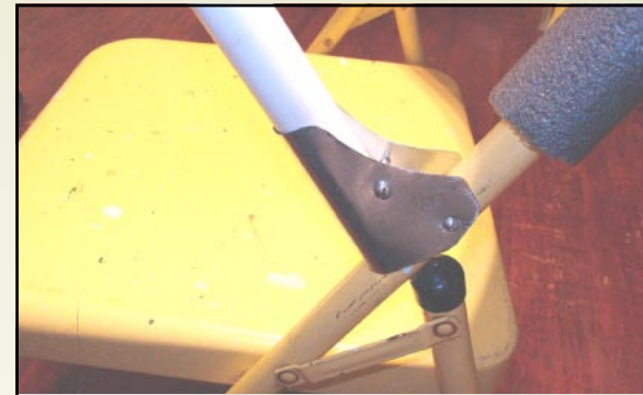
Figure 3. Bolt Bracket To Chair and PVC Pipe To Bracket
