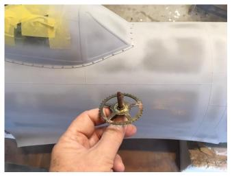
I then got out my special rivet tool from the north production plant. A run along each panel line and I have simulated flush rivets.
