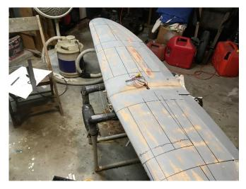
This pic shows the wing with the panel lines al taped up. I used 1/16" chart tape and I sprayed over with primer.
