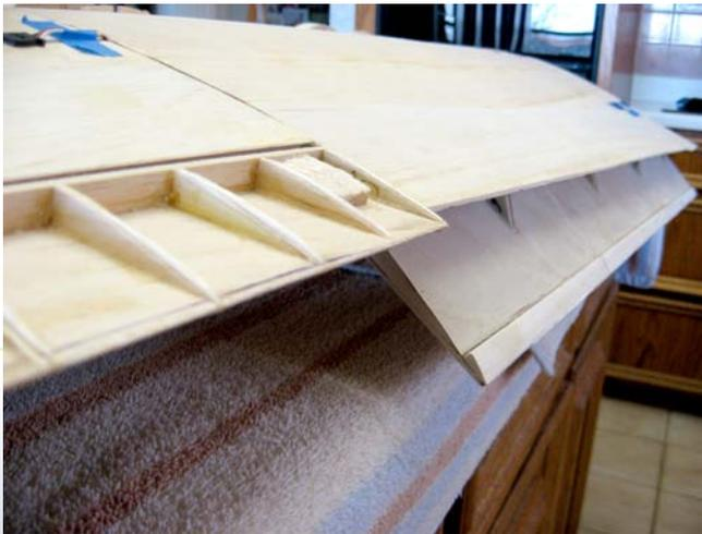
The last picture shows one of the two intermediate Fowler flap hinges in its installed position. The small rods shown are the smooth portion of a #2-56 control rod.
