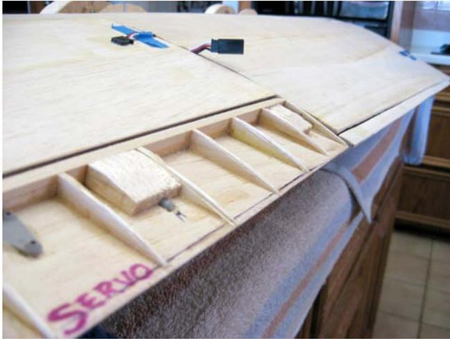
The photo to the left shows the B-24 port wing, looking from the tip toward the root. The frame is in the bones, and the aileron is shown in the foreground, with the completed flap on the wing in the up position.
