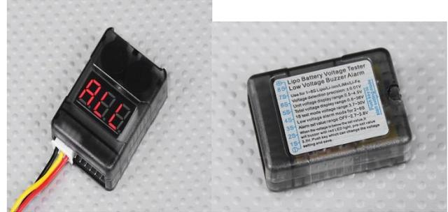
All you do is plug your balance tap of your battery into the checker and it will read the voltage of each cell, up to 8 cells. You can also leave this unit plugged into your battery in flight and it will warn you by beeping when it gets to the target voltage. Some are louder than others so the plane has to be pretty close to you to hear it. Just make sure the black wire is to your far left and it will figure out how many cells you have.
