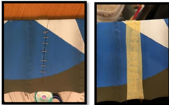
Now this is the bottom wing that 2/3's of it was GONE. I spliced the spars into the existing wing and built the other half. I have all the covering for the wing and the aileron intact. So, in the next week I will build the center cabane struts and then start re-covering with all the existing covering. Here again I am shooting for first of March.
