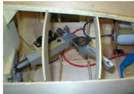
This is a pic of the nose gear installation. Instead of using a pull pull cable system for the steering servod, I just drilled and tapped a servo mount on the nose gear arm. As I said before, “In theory they should work”.
